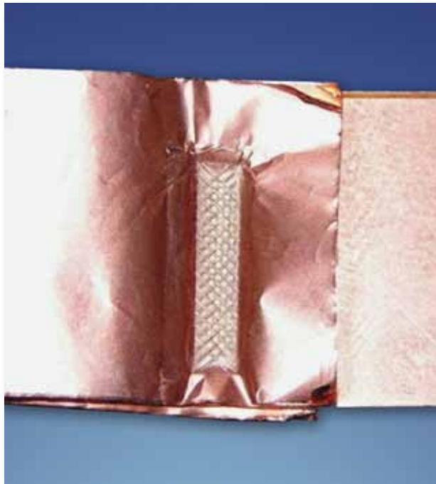
Ultrasonic metal welding technology provides a cost-effective, environmentally friendly method for attaching multiple layers of foil to tabs and terminals used in lithium-ion and NiMH battery assembly. Up to 100 layers of copper and aluminum foils as thin as 7 \mu\text{m} can be welded without tearing, and in just one pulse.
